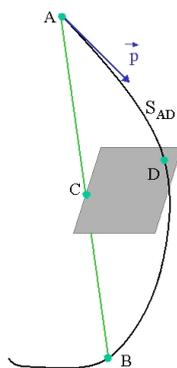
**Figure 4.7.** The distance between the calculated chord intersection point C and a computed curve point D is used to determine whether C is an accurate representation of the intersection of the curved path ADB with a volume boundary. Here CD is likely too large, and a new intersection on the chord AD will be calculated.
